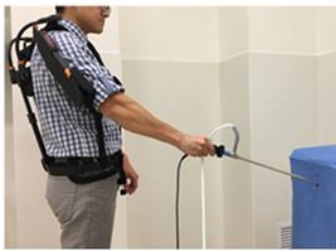
Fig. 4 Laparoscopic camera holding test. Subjects are asked to point to a painted target about 3 ft away
